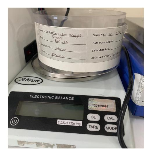
Analytical balances are precision measuring instruments used in quantitative chemical analysis, to determine the mass of solid objects, liquids, powders and granular substances.
