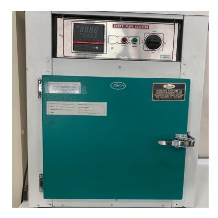
A hot air oven is a type of dry heat sterilization. Dry heat sterilization is used on equipment that cannot be wet and on material that will not melt, catch fire, or change form when exposed to high temperatures. Moist heat sterilization uses water to boil items or steam them to sterilize and doesn't take as long as dry heat sterilization. Examples of items that aren't sterilized in a hot air oven are surgical dressings, rubber items, or plastic material.
