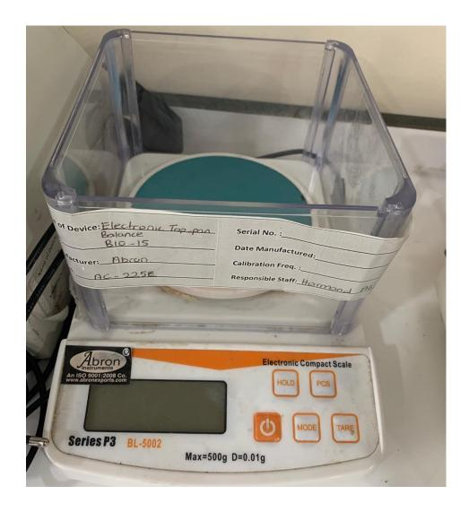
The term *Top Pan Balance or Top Loading Balance* refers to weighing scales and balances that have a pan that is not enclosed by the body of the machine. Top pan balances commonly attach the weighing plate to the top of the balance and relates to machines that have a resolution not requiring a draft shield to protect the weighing surface.
