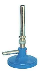
A Bunsen burner is a type of gas burner commonly used as a heat source in laboratory experiments. The burner consists of a flat base with a straight tube extending vertically, known as the barrel or chimney. Natural gas (predominantly methane) or a liquified petroleum gas such as propane or butane is supplied at the bottom of the chimney.
