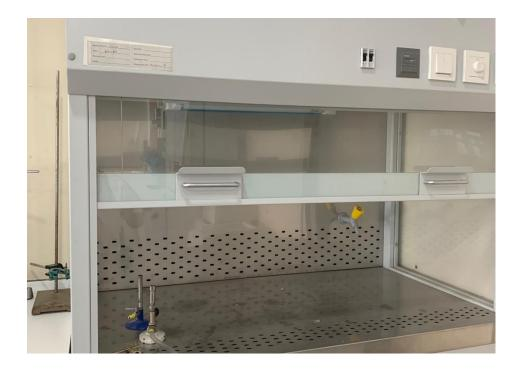
Fume hoods are a form of regulation in environments that are exposed to harmful vapors and fumes. In order to protect people from the harmful effects of these fumes, fume hoods are used to get rid of the harmful aspects and allow the individuals to work safely. Labs use fume hoods when working with substances that let off a harmful fume or odor. Laboratory workers can work with substances directly under the fume hood, or simply place the substance in the fume hood after the work is done.
