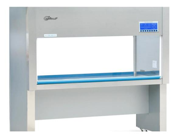
A laminar flow cabinet is defined as enclosed workbench which is used to create a contamination free work environment through installed HEPA filters that capture all the particles entering the cabinet. A laminar flow hood is used for work with substances which are not hazardous for the personnel health.
