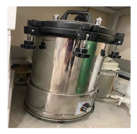
Autoclaves are also known as **steam sterilizers**, and are typically used for healthcare or industrial applications. An autoclave is a machine that uses steam under pressure to kill harmful bacteria, viruses, fungi, and spores on items that are placed inside a pressure vessel. The items are heated to an appropriate sterilization temperature for a given amount of time. The moisture in the steam efficiently transfers heat to the items to destroy the protein structure of the bacteria and spores.
