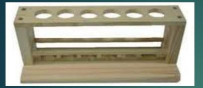
Test tube racks are pieces of equipment that are used to hold upright multiple test tubes at the same time
