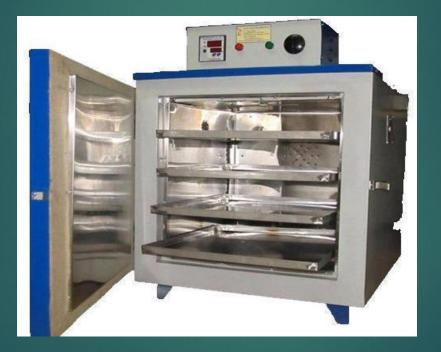
For routine purpose, sterilization can be achieved by running the equipment at 180°C for 1.5 hours. Hot air oven is less effective than autoclave 4. Inoculating loop This is a tool for transferring and streaking cultures Inoculating needles are used for preparing 'stab' cultures
