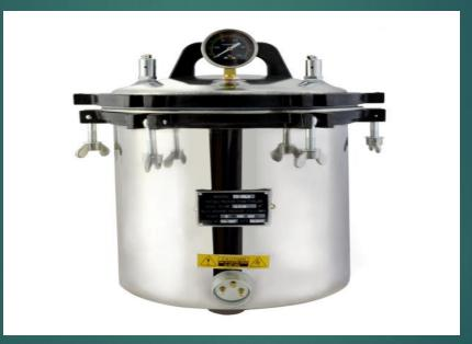
In routine process, sterilization can be achieved by operating the autoclave at 121°C (15 psig) for 15 min.
