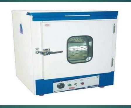
For routine purposes, the temperature is maintained at 28-30°C for bacteria, about 25°C for molds, and 35-37°C for mesophilic bacteria. A temperature as 2 high as 100°C can also be maintained for extremely thermophilic organisms (stereothermophiles)
