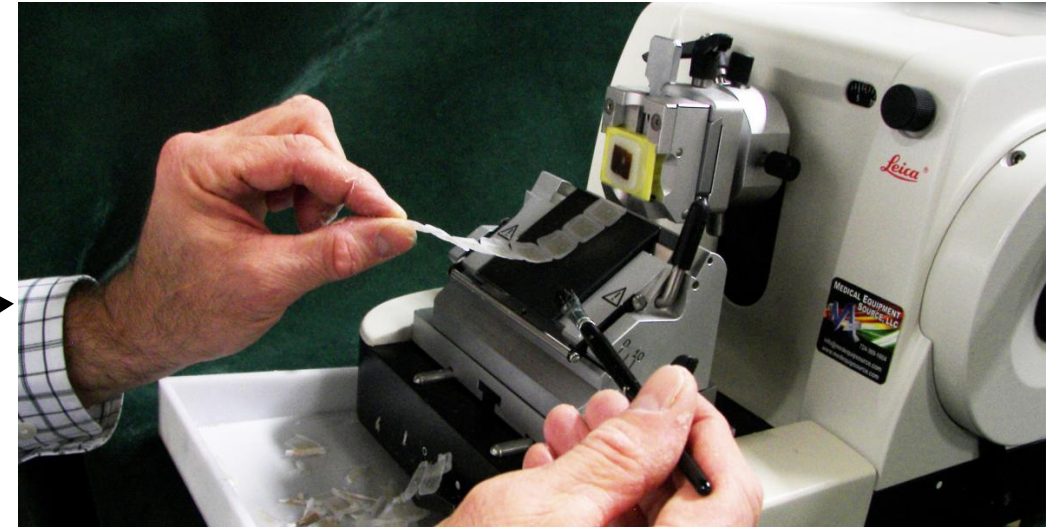
Cutting sections using microtome
